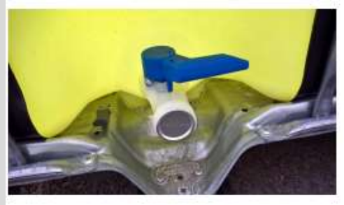
Figure 2. Sealed openings on the bottom of bulk packaging
