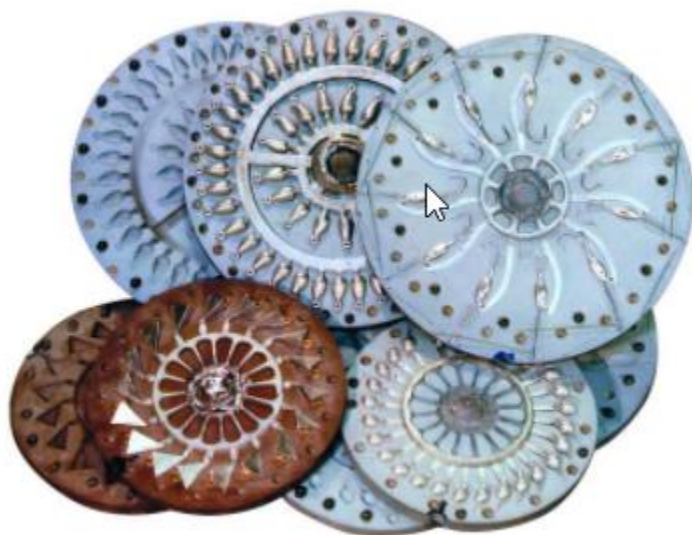
Figure A.2-9 Spin casting mould to manufacture jigs or jig-heads.
