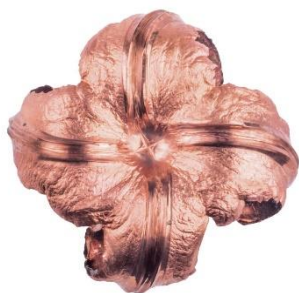
Figure D.1-13: Barnes TSX, TTSX, MRX expanded. Picture Federal Cartridge Co.
