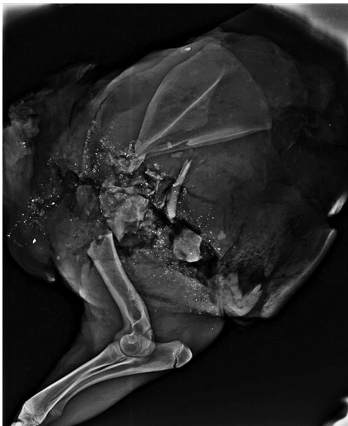
Figure B.9-9 X-Ray image of a wild boar skull where a conventional, bonded bullet hit the upper arm bone and severely fragmented (Swedish NFA, 2014a)
