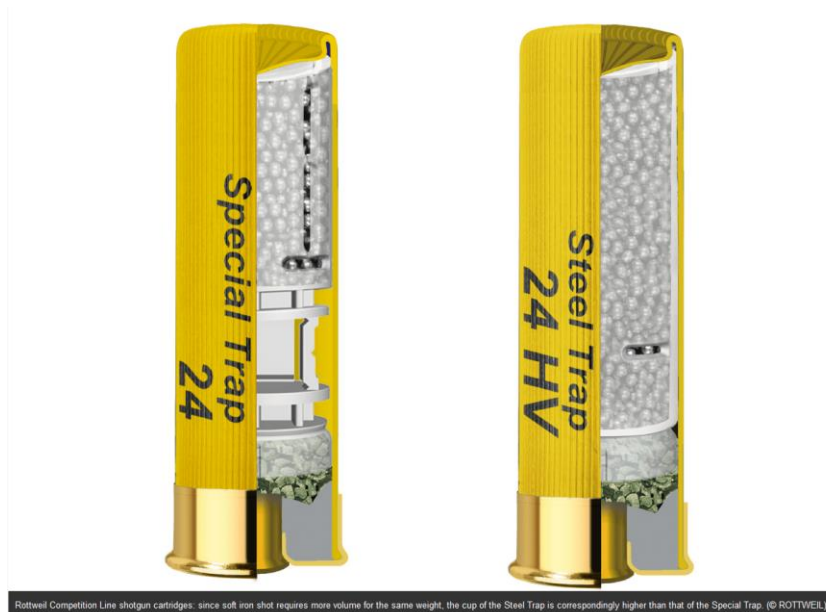
Figure C.1-1 Rottweil Competition Line shotgun cartridges with lead shots (left) and soft iron shots (right)
