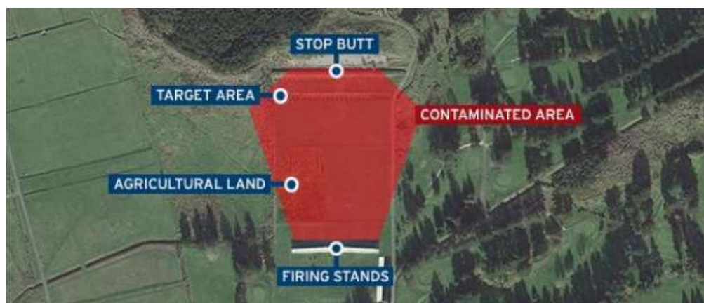
Figure 1-27: Example of lead deposition on agricultural land from a rifle/ pistol range (Environmental Protection Authority Victoria (EPA), 2019)
