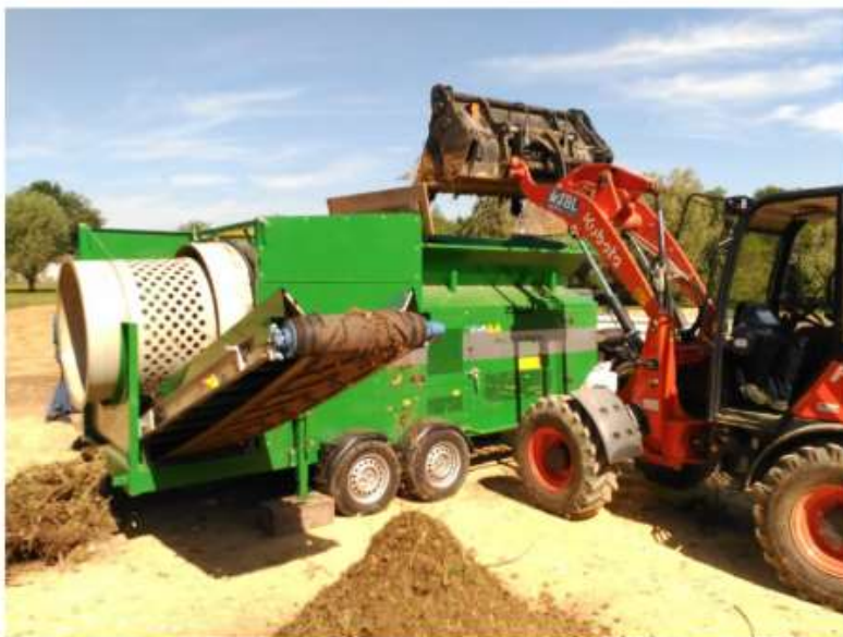
Figure 1-2: Two examples of large screening machines used for mechanical intervention on level ground (FITASC/ISSF comment #3221)
