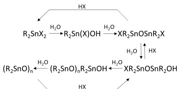
Figure: Hydrolysis scheme for dialkyltins (Davies, 2004; Aylett *et al.*, 1979)
