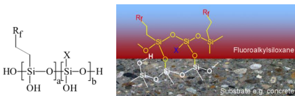
Structural formula and model of a water-based fluoroalkylsilane system. R f are fluoroalkyl groups and X are hydrophilic groups (Standke et al. , year not indicated)
