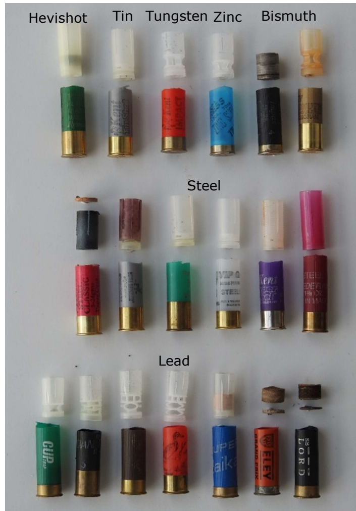
Figure E-10. Wad construction in a selection of shotgun cartridges. All calibre 12. Bottom: Lead; Middle: Steel; Top (from left): Hevishot, Tin, Tungsten, Zinc and two Bismuth. See text for details.
