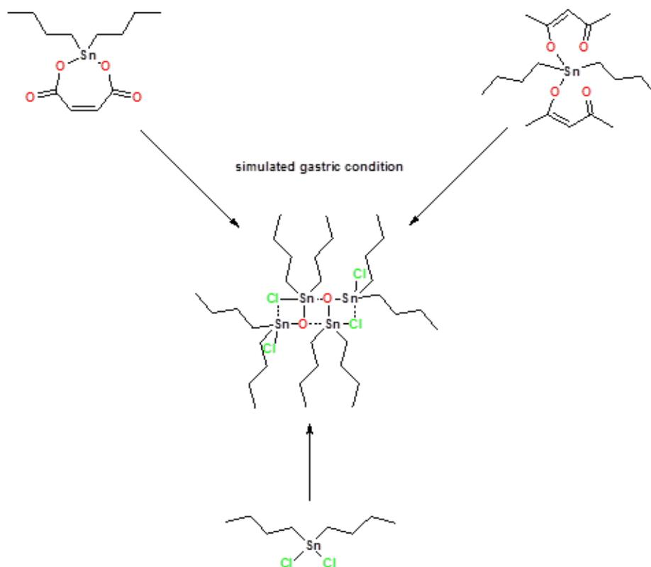
**Figure 3. Overview of the hydrolysis of DBTM, DBTP and DBTC as determined in recent studies (Naßhan, 2015, 2016, Umweltbundesamt, 2019), which is in accordance with well established tin chemistry (Davies, 2004; Aylett et al., 1979).**
