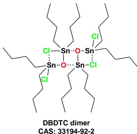
**Figure 1: Dimer distannoxane (ClBu<sub>2</sub>SnOSnBu<sub>2</sub>Cl)<sub>2</sub>**
