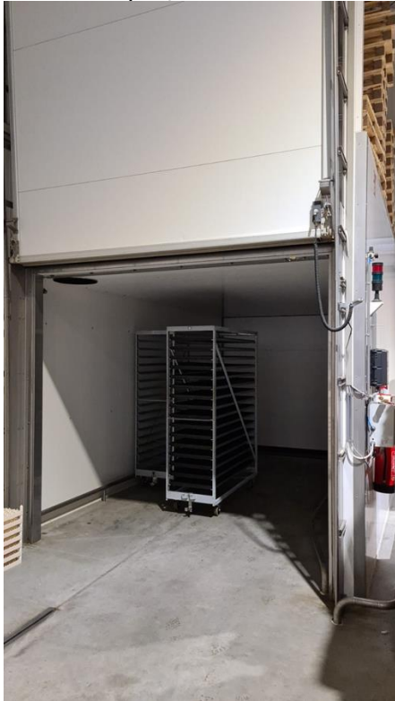
Figure 1: Example of a disinfection sluice
