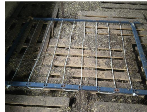
J15' polyethylene'rods'treated'with'master' batch'9028'PE'Anti'rodent'at'2'%'
