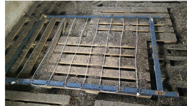
J21' polyethylene'rods'treated'with'master' batch'9028'PE'Anti'rodent'at'2'%'
