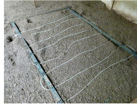
J56' Terrarium'12' polyethylene'rods'treated'with'master'batch'9028'PE' Anti'rodent'at'2'%'
