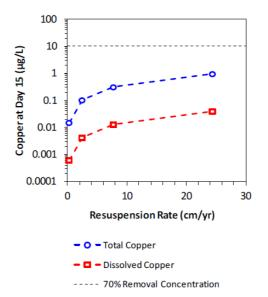
Figure 4. Effect of resuspension rate on total and dissolved copper concentration at day 15 in oxic sediment
