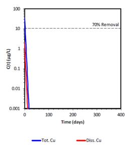
Figure 8. TICKET-UWM simulations with water column isolated from the sediment (i.e., no feedback/remobilization) for initial total copper equal to 35  $\mu$ g/L. The dashed line is at a concentration corresponding to 30% remaining (70% removal) based on the initial total concentration.
