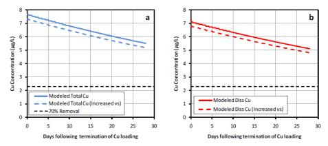
Figure 13. a) Total and b) dissolved copper TICKET-UWM results from post-loading simulations for the observed  $K_{\rm D}$  and settling velocity scenario. Model simulations use the experimentally-estimated values for the water column  $K_{\rm D}$  (104.12 L/kg) and settling velocity (0.2 m/d). The blue and red dashed lines refer to simulations with the settling velocity increased to 0.28 m/d. The horizontal black dashed line denotes 70% copper removal.
