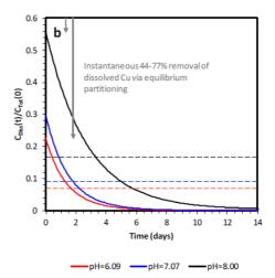
Figure 3. a) Dissolved and b) total copper removal from the water column under different pH conditions for a DOC concentration of 15 mg/L. Copper speciation (including binding to POC) was calculated using WHAM V in TICKET-UWM. The initial total copper concentration in the water column, CTot(0), was set at the pH-specific acute ERV (Table 2-1). The horizontal dashed line represents C(t)/CTot(0) = 0.3 or 70% removal of copper.
